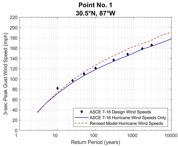
**Figure 3-2. Predicted peak gust wind speeds at a height of 10 m at 30.5°N, 87.0°W.**
