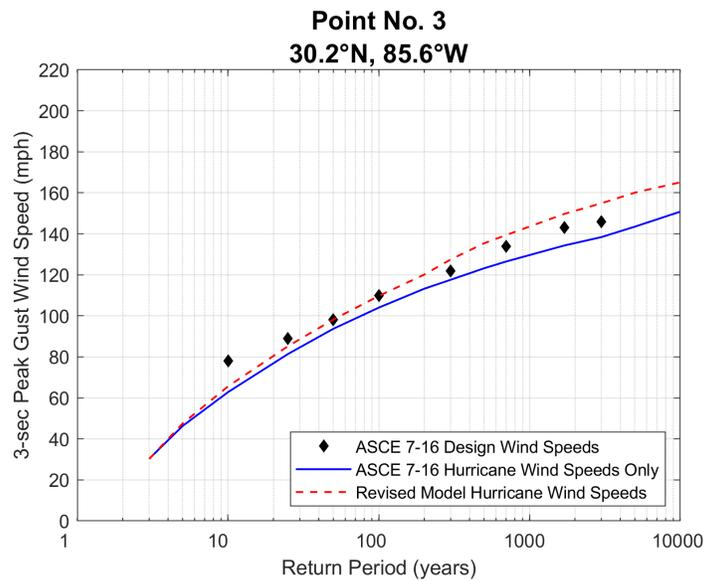
**Figure 3-4. Predicted peak gust wind speeds at a height of 10 m at 30.2°N, 85.6°W.**
