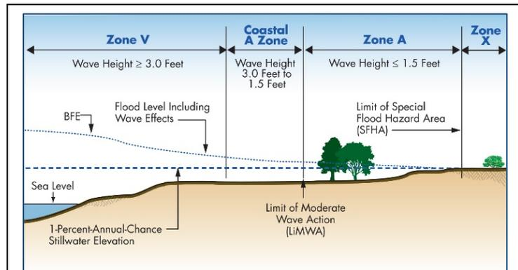
Figure 5. Schematic coastal cross section.
