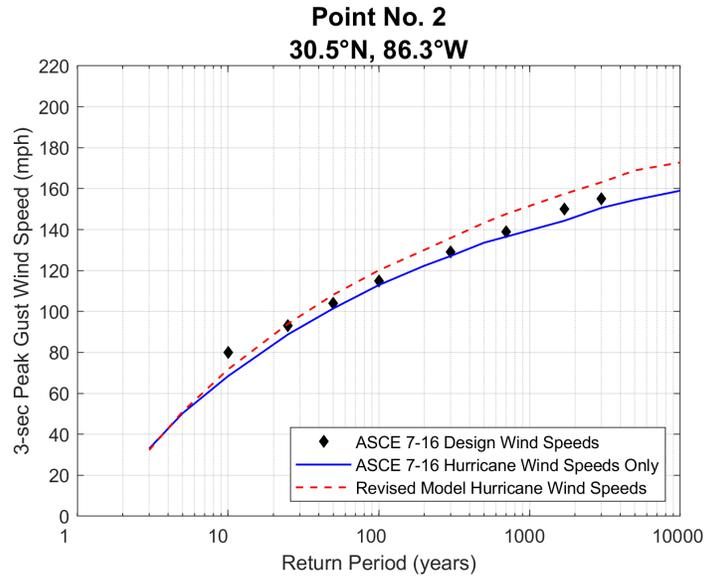
**Figure 3-3. Predicted peak gust wind speeds at a height of 10 m at 30.5°N, 86.3°W.**
