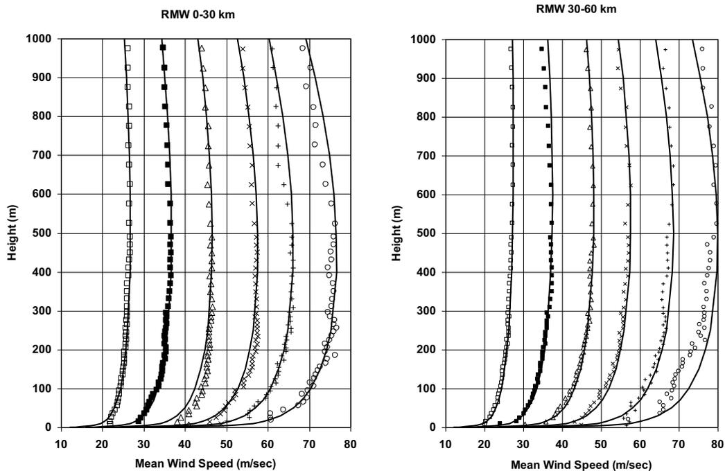
**Figure 2-7. Modeled and observed hurricane mean vertical profiles of horizontal wind speed over the open ocean for a range of mean wind speeds**
