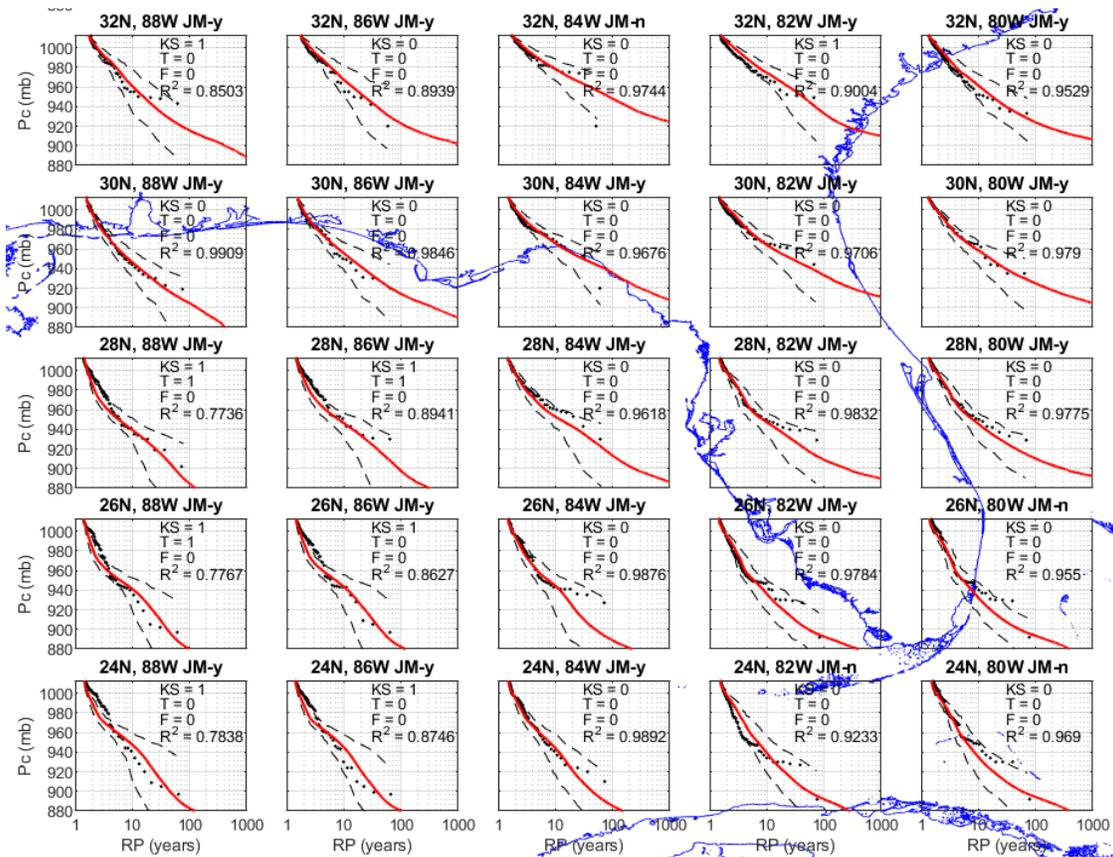
**Figure 2-6. Modeled and observed central pressures vs. return period for points located near Florida. JM = n indicates failure of the empirical distribution equivalence test proposed by James and Mason (2005). F=1 indicates failure of F-test, T=1 indicates failure of the t-test, KS=1 indicates failure of the KS test. Dashed lines represent the 95% confidence interval.**
