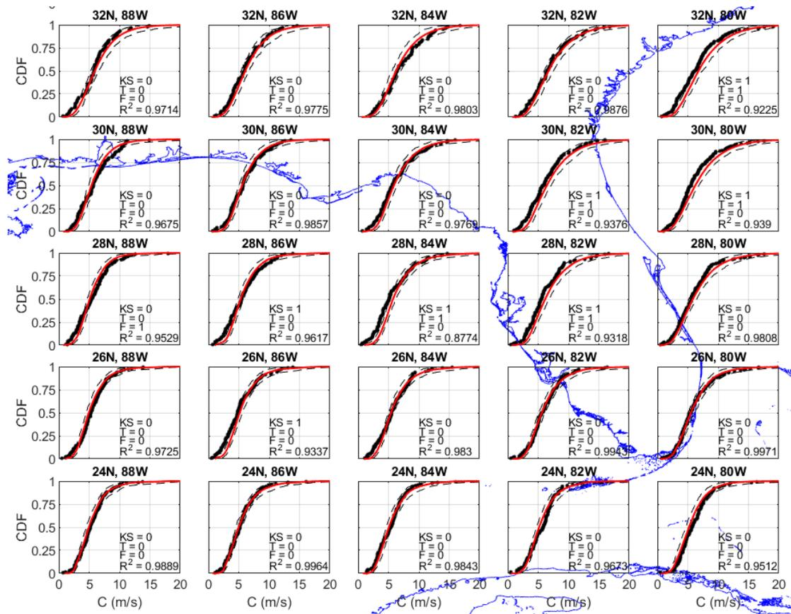
Figure 2-4. Comparisons of modeled and observed CDF's of storm translation speed for locations near Florida. F=1 indicates failure of F-test, T=1 indicates failure of the t-test, KS=1 indicates failure of the KS test. Dashed lines represent the 95% confidence interval.
