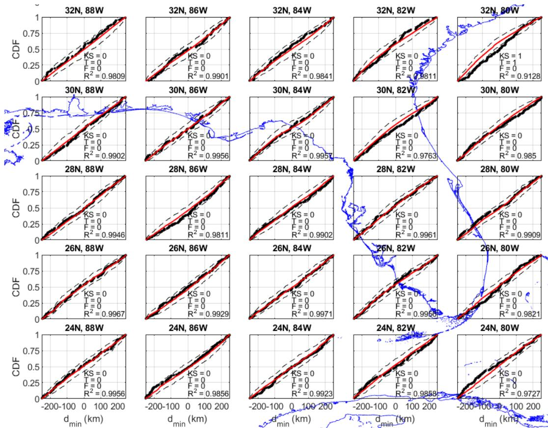
**Figure 2-5. Comparisons of modeled and observed CDF's of distance of closest approach for locations near Florida. F=1 indicates failure of F-test, T=1 indicates failure of the t-test, KS=1 indicates failure of the KS test. Dashed lines represent the 95% confidence interval.**
