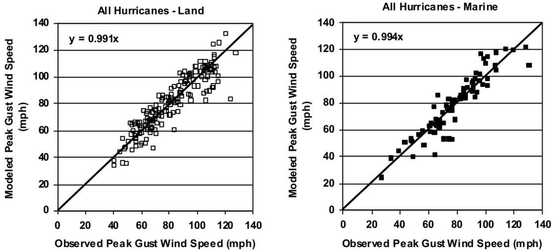
**Figure 2-9. Example comparisons of modeled and observed maximum surface level peak gust wind speeds from landfalling hurricanes. Wind speeds measured on land are given for open terrain and wind speeds measured over water are given for marine terrain.**
