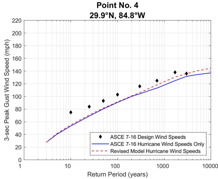
**Figure 3-5. Predicted peak gust wind speeds at a height of 10 m at 29.9°N, 84.8°W.**
